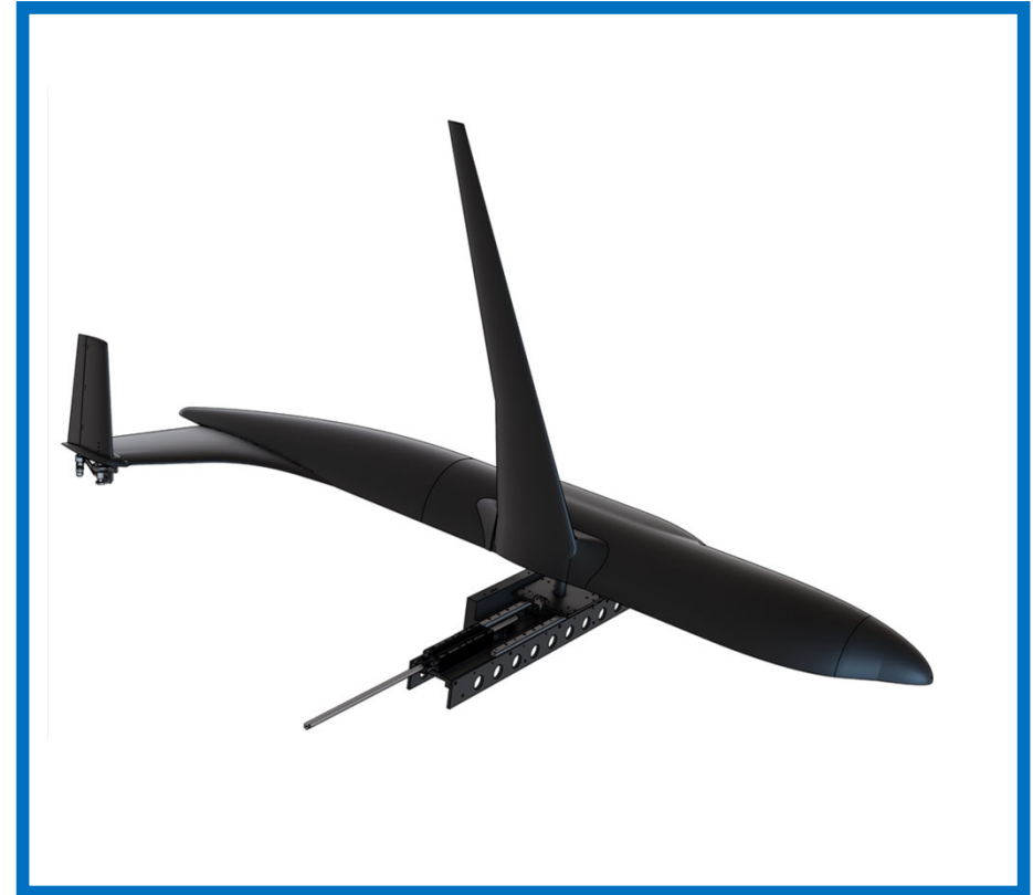
Aeroelastic FWT half model AE2 To Be Tested @ POLIMI
