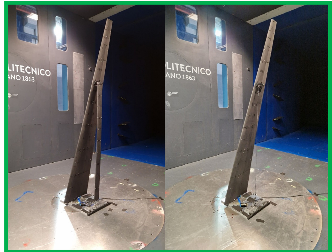
Aeroelastic SBW wing model AE1 Tested @ POLIMI
